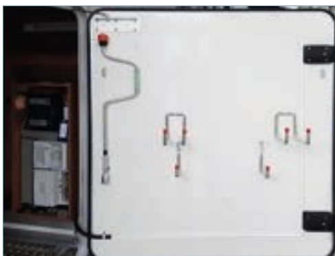
Installation example: Carthago C-Line semi-integrated Cable ducts on the rear flap.
