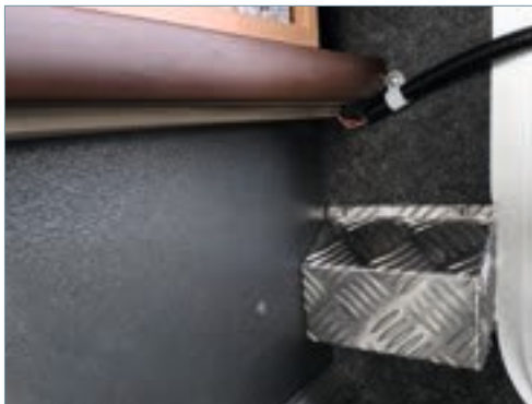
Installation example Carthago C-Line/C-Tourer The two rear garage flaps are connected by cable via the brown cable duct.
